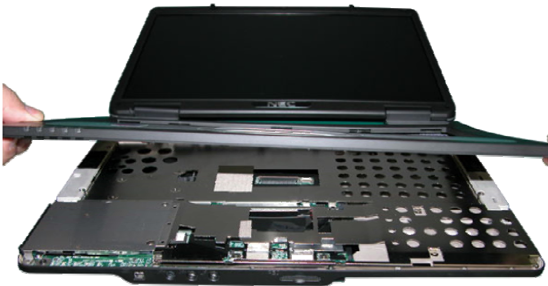
Fig. 20 Removing the Top Cover
